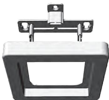
The wall mounting plate is either mounted to the wall using three screws or affixed to the bottom of the mounting box. The mounting plate is covered first with a cover plate and finally with the control panel. The length of the sensor cable is 8 m. Cut the excess wire and connect the other end to the heater. When installing the control panel, make sure that the cables do not become detached or bend.
